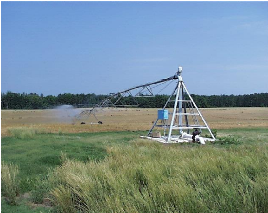
Figure 10-5. Center pivot system.
