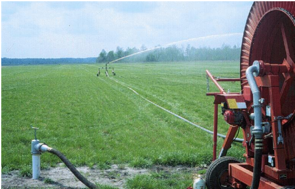
Figure 10-3. Hard hose traveler showing reel and gun cart.
